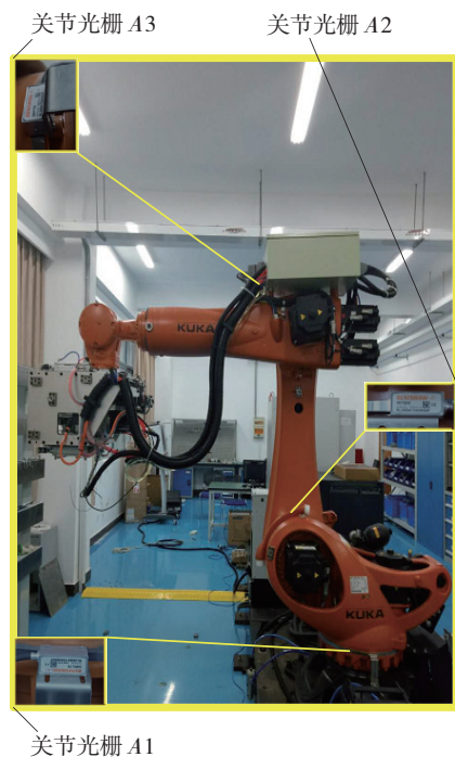
图2 机器人关节光栅的安装 Fig.2 Installation of robot joint grating
