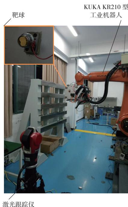
图3 激光跟踪仪和靶球的相对位置 Fig.3 Laser tracker and SMR (Spherically Mounted Reflector)
